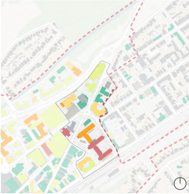
Fig 83 Existing heights by building
