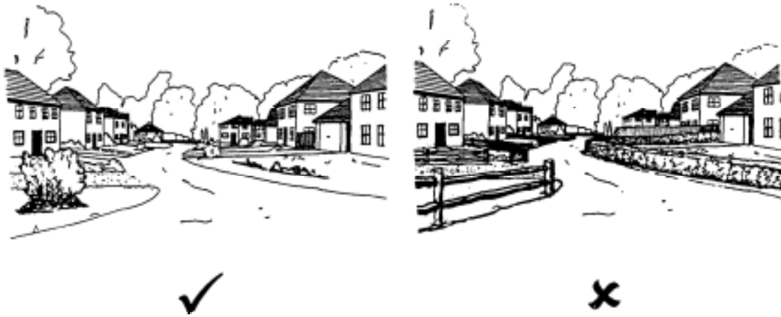
Figure 7: The enclosing of front gardens on an ‘open plan’ estate with walls and fences will completely change the character of the street scene and are discouraged.
