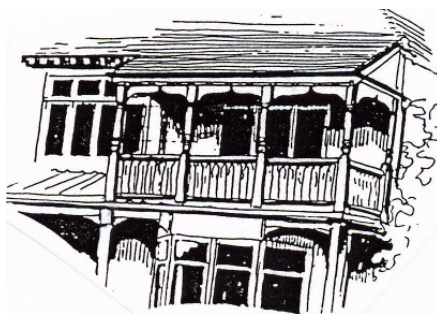
A typical partly enclosed loggia
