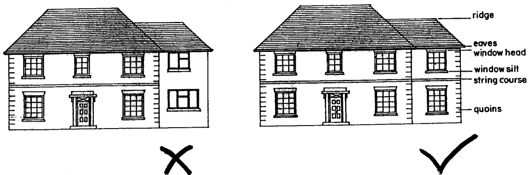
Fig. 3 Elevational detail should closely match that of the existing dwelling.
